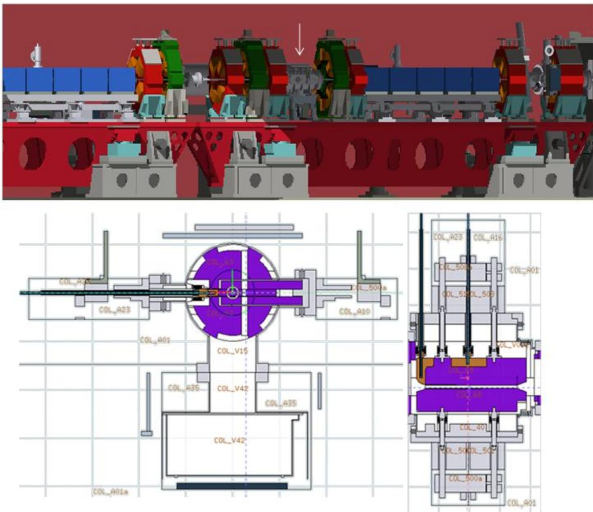
*Fig.2 – FLUKA model of the beam loss collimator. Top: part of the beam loss collimator cell. Bottom: left: vertical section; right: horizontal section.*
