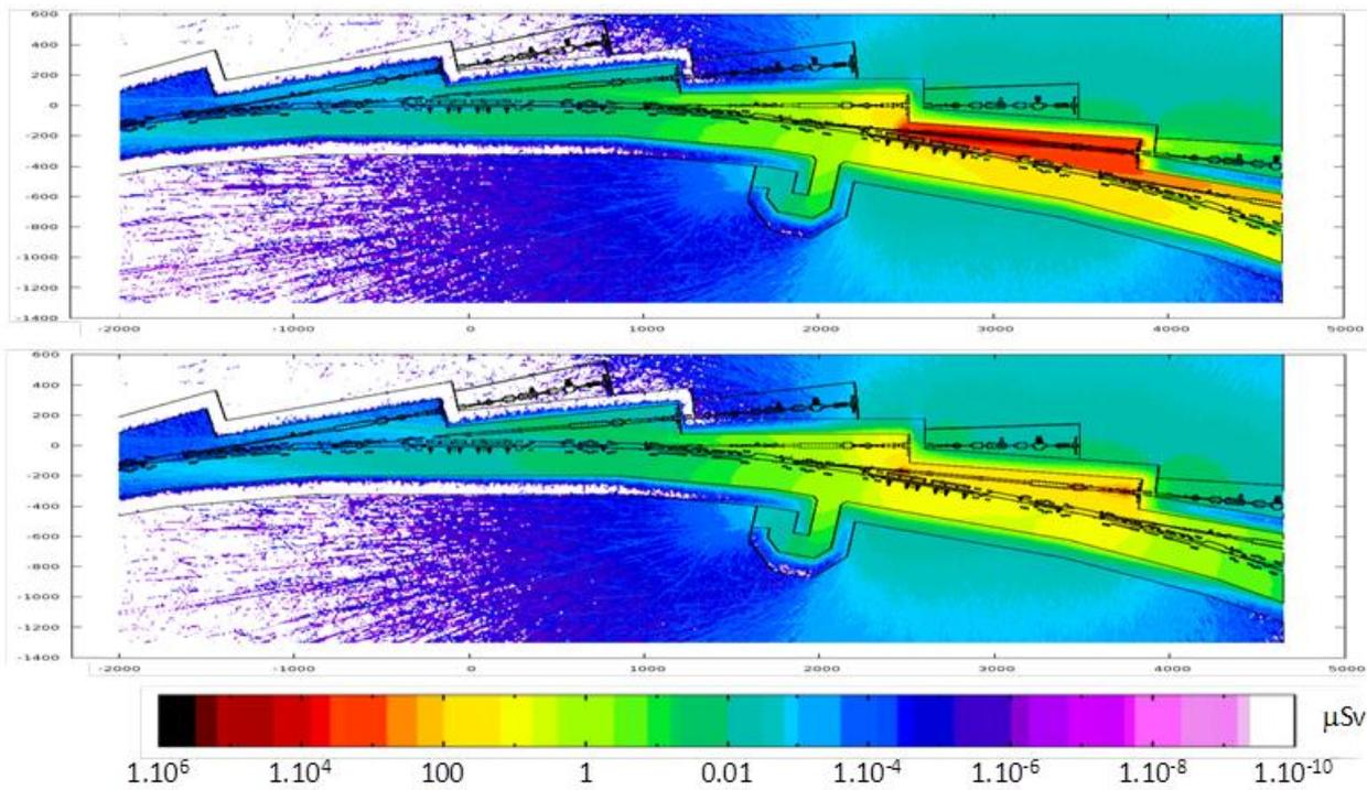
*Fig.5 – Integrated effective dose distribution from a 5 nC pulse from the booster lost due to zero field in the DQID magnet in the central unit cell. Dose distribution in horizontal plane at beam height. Top: total dose – Bottom: neutron dose. Dimensions in cm.*
