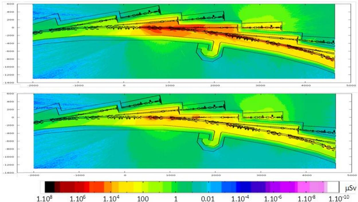
*Fig.4 – Integrated effective dose distribution due to 200 mA beam loss caused by closing of 1<sup>st</sup> gate valve in the central unit cell. Dose distribution in horizontal plane at beam height. Top: total dose – Bottom: neutron dose. Dimensions in cm.*
