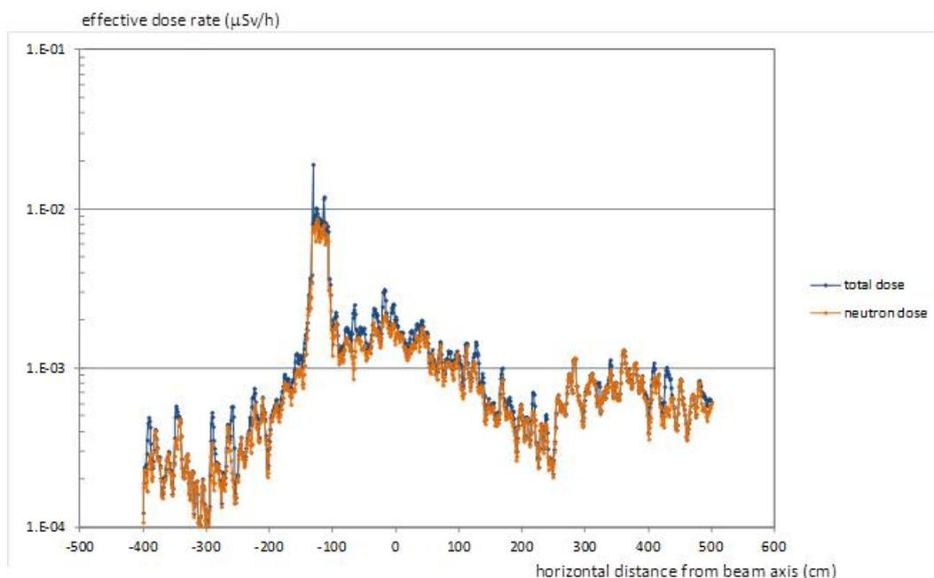
Fig.6 – Total and neutron effective dose rates above the storage ring tunnel roof, averaged over the length of the RF duct, as a function of the horizontal distance from the beam axis. 92 mA, 1.8 h lifetime beam decay.
