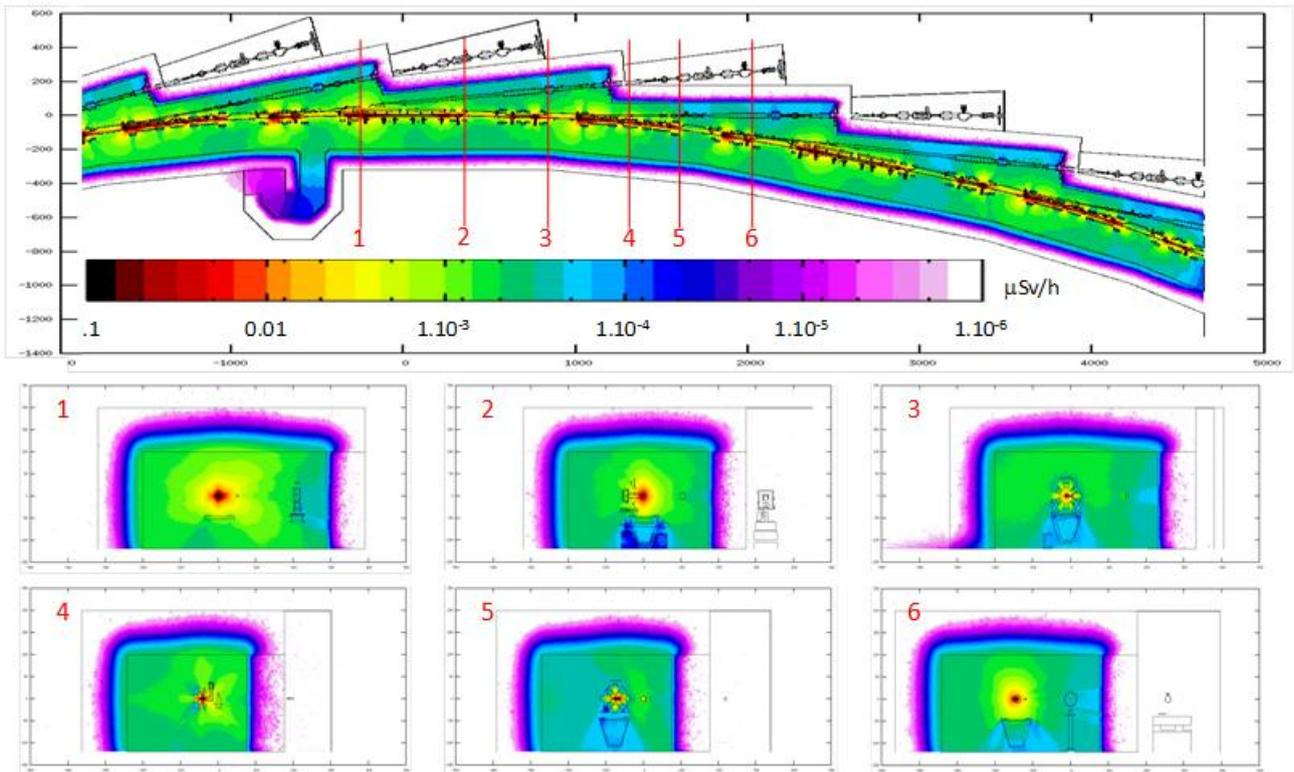
Fig.8 – Residual effective dose rates inside the storage ring tunnel cells 19, 20 and 21, for a 1 day decay period, after 21 years of operation. Top: effective dose rates in horizontal plane at beam height. Bottom: effective dose rates in 6 selected vertical planes.
