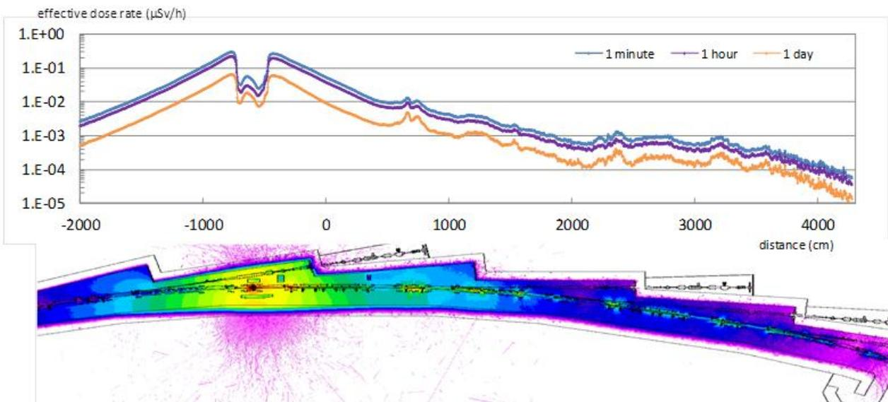
Fig.8 – Residual effective dose rates at 1 m from the beam axis (walkway) rates inside the storage ring tunnel around the beam loss collimator, for 3 different decay periods (1 minute, 1 hour and 1 day respectively), after 21 years. Dose rates given in horizontal plane at beam height.
