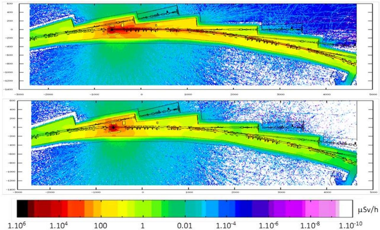
*Fig.3 – Effective dose rate distribution around the collimator in cell 13 during a 92 mA, 1.8 h lifetime stored beam decay. Dose distribution in horizontal plane at beam height. Top: total dose – Bottom: neutron dose. Dimensions in cm.*
