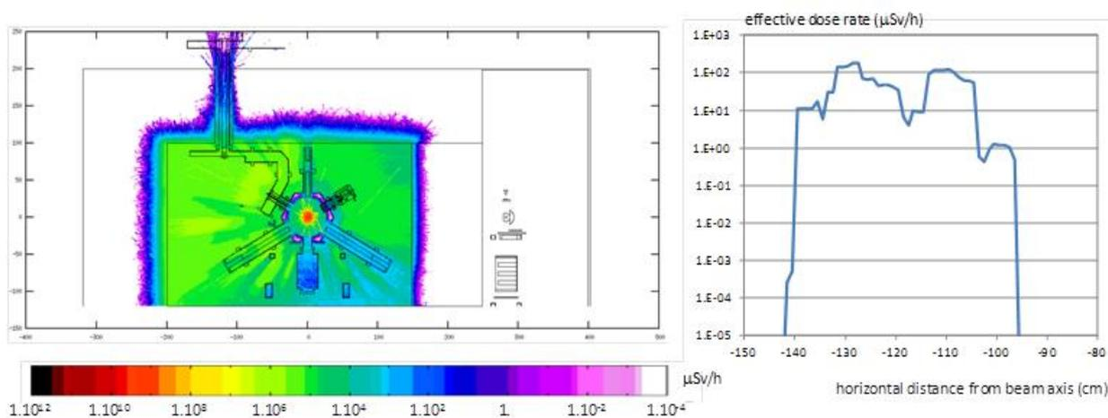
Fig.7 – Synchrotron radiation effective dose rates through one of the RF ducts. Left: dose distribution in vertical plane, averaged over duct. Right: effective dose rates on top of the roof as a function of the horizontal distance from the beam axis. Conditions: 200 mA stored beam.
