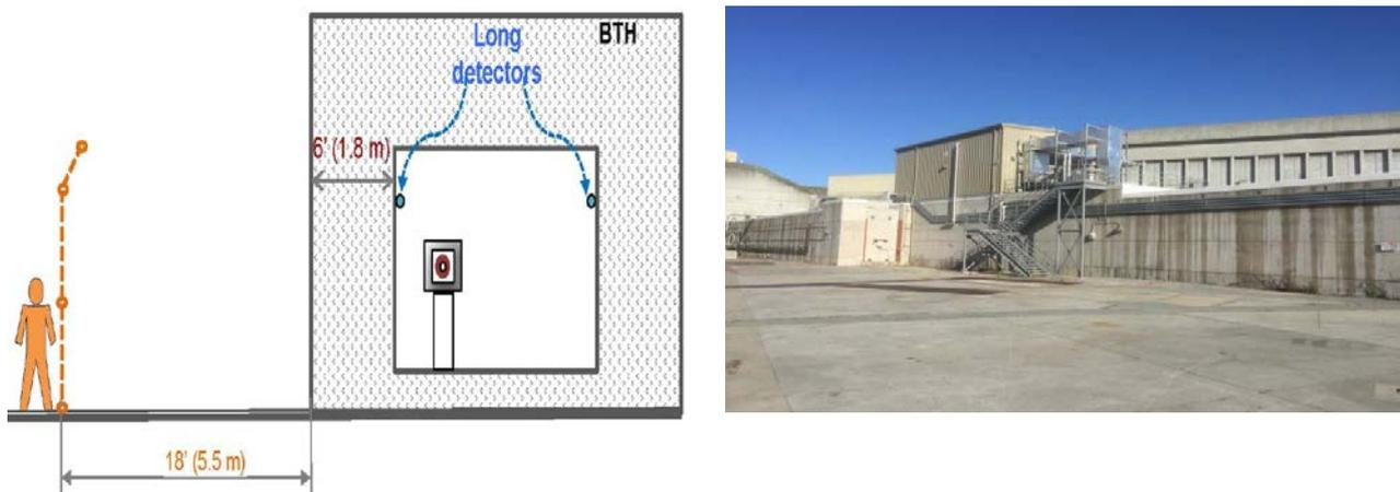
Fig.2 – (L) Schematic of LCLS Beam Transport Hall (BTH) designed for 5 kW. Fence will be added for LCLS-II operations; (R) photo of BTH- 2x120 kW beams will be transported from left to right
