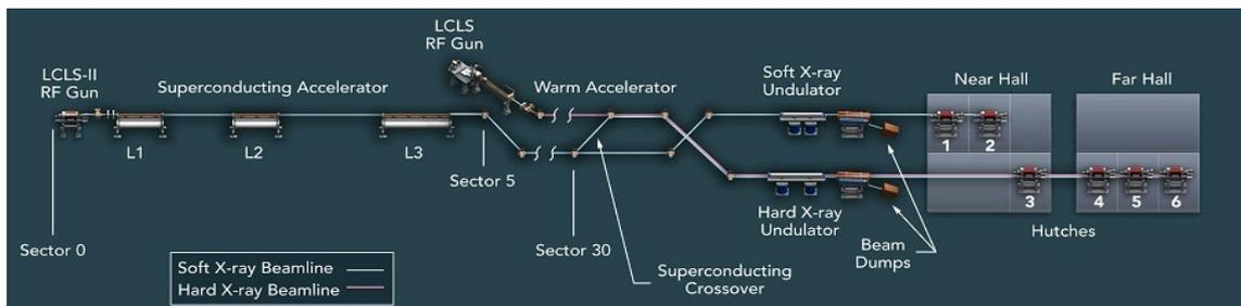
Fig.1 - Schematic of SLAC linear accelerator facility including the layout of the new LCLS-II accelerator
