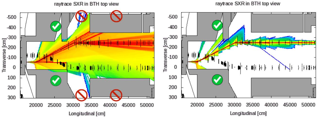
Fig.3 – (L) ray-trace studies for the LCLS-II beam in SXR (without protection collimators); (R) ray-trace studies for the LCLS-II beam in SXR (with protection collimators)
