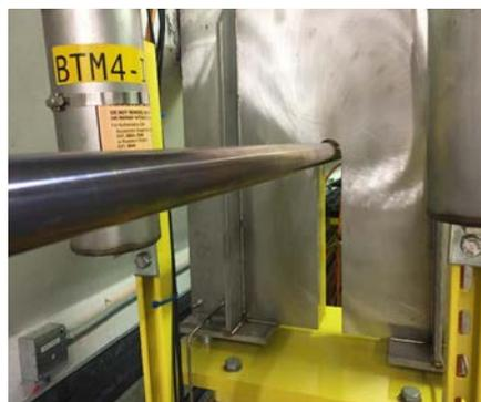
Fig.4 –Protection Collimator, Burn Through Monitor and Ion Chamber deployed in LCLS
