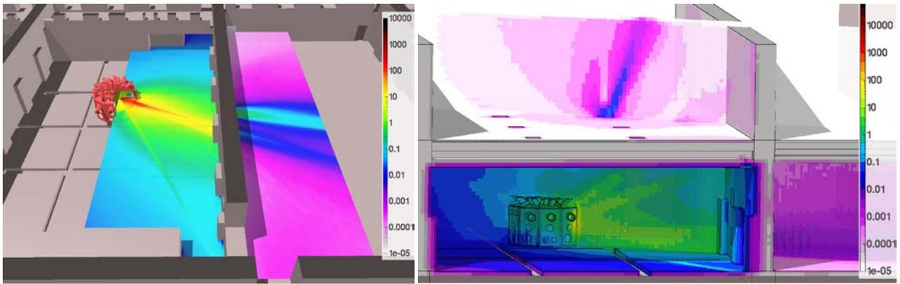
Fig.2 –  $H^*(10)$  rate map [mSv/shot] for P3 beamline, solid target experiment, complex source term ( $\gamma$ ,  $p$ ,  $e^+$ ,  $e^-$ ). Horizontal (left) and vertical (right) plane.
