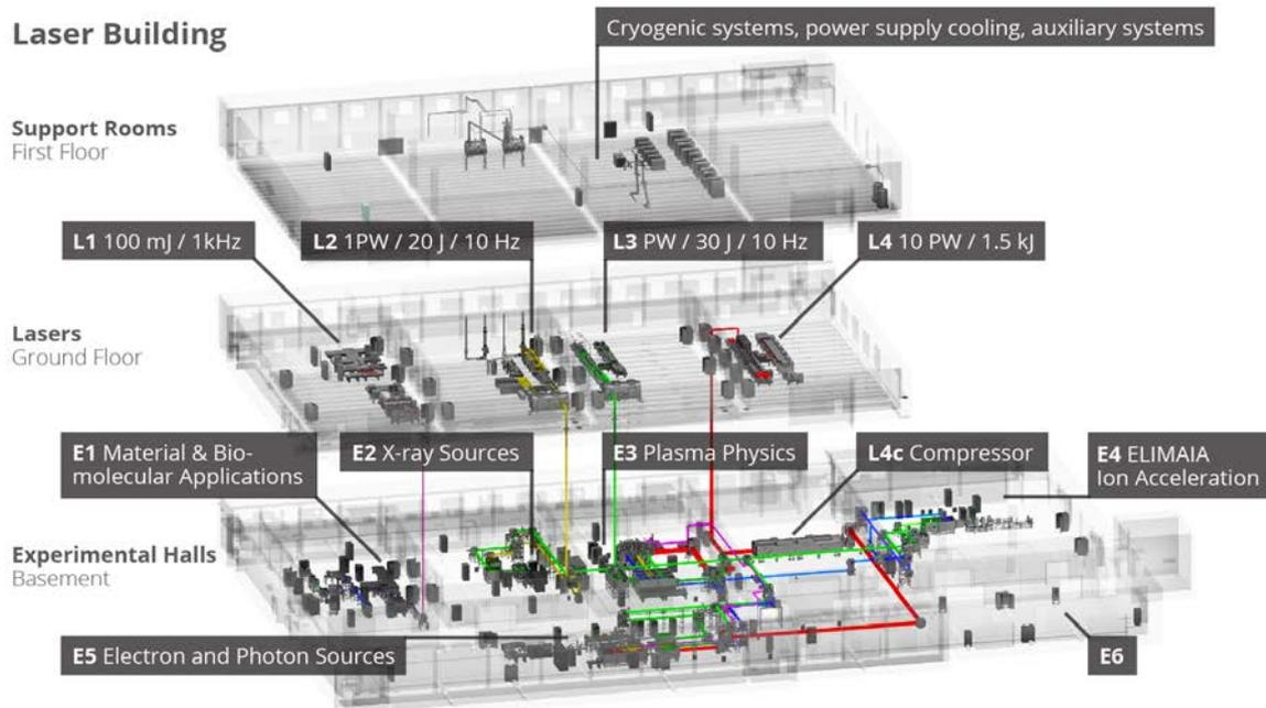
Fig.1 – Scheme of ELI Beamlines experimental building
