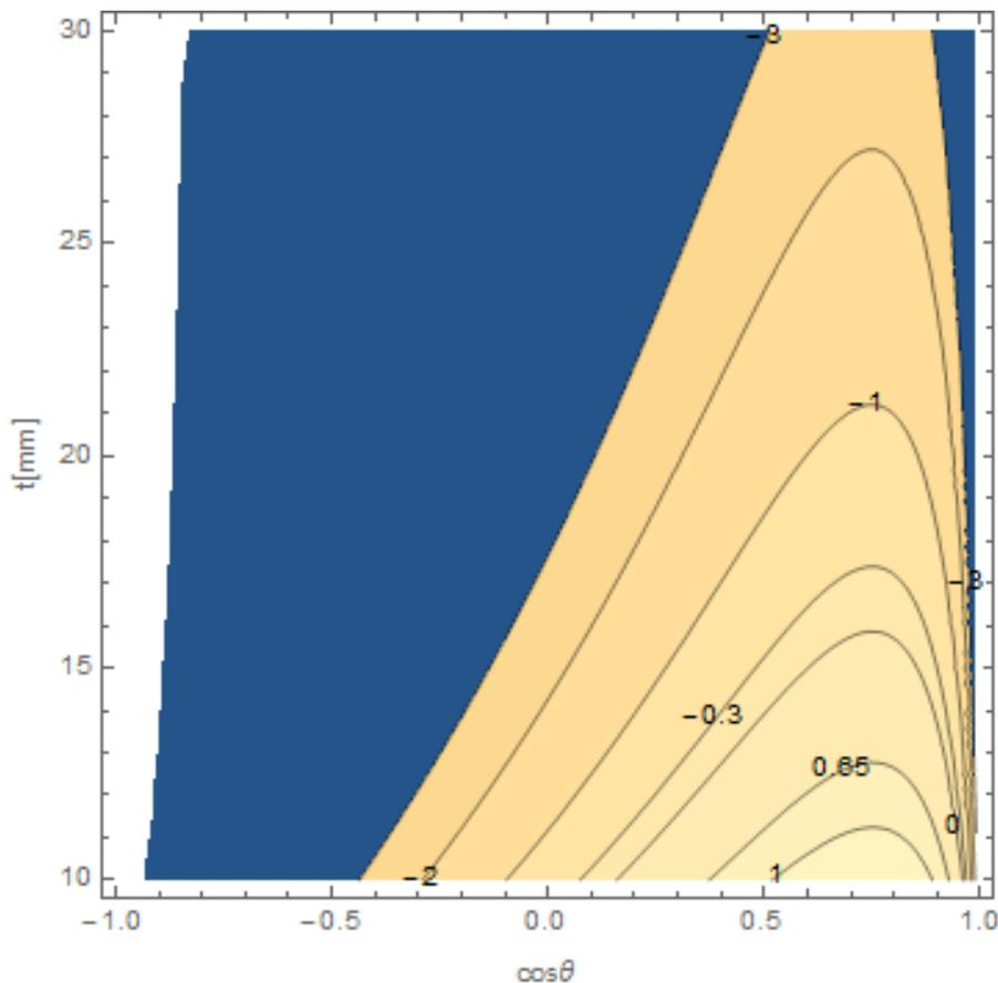
Fig.6: Dose rate as function of lead thickness and scattering angle for a beam size of  $9\text{mm}^2$  and a distance of  $1\text{m}$  from the target.
