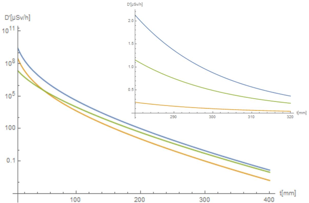
Fig.3: Dose rate due to scattering as function of wall thickness (equal to distance from target) for white radiation (yellow: beam size 1mm<sup>2</sup>, blue: beam size 9mm<sup>2</sup>, green: beam size 9mm<sup>2</sup> but with 100mm additional distance to target)
