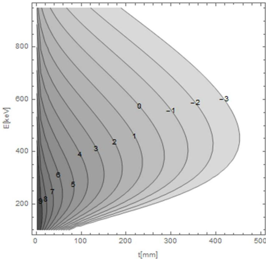
Fig.2: Common logarithm of the dose rate per 1keV energy band in units of  $\text{nSv/keV/h}$  as function of energy and wall thickness. The shift to higher energies is due to beam hardening with increasing shielding thickness.
