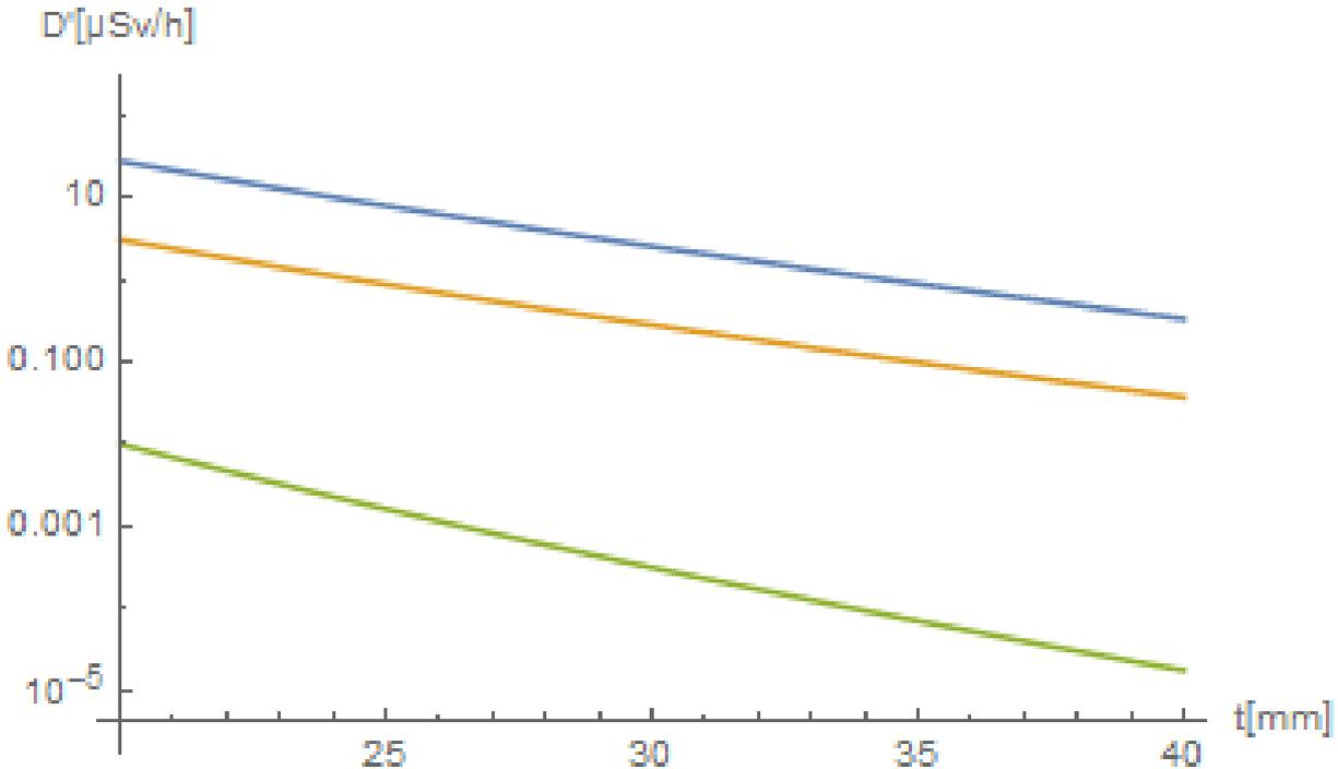
Fig.5: Dose rate as function of lead thickness for forward scattering and 1m distance from the target. (green: standard undulator, yellow and blue: P61 wiggler 1mm<sup>2</sup> and 9mm<sup>2</sup> beam size respectively)
