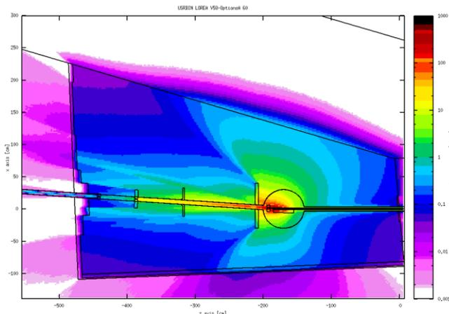
Fig. 2 - Photon dose rate map (in  $\mu\text{Sv/h}$ ) from scattered bremsstrahlung
