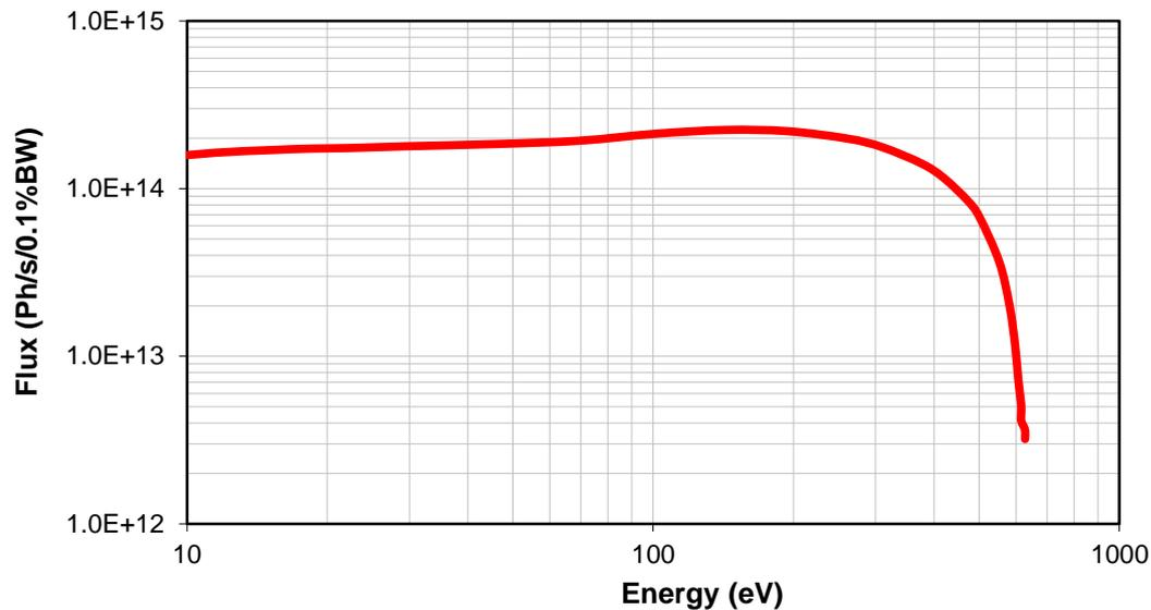
Fig. 6 – LOREA ID Undulator photon flux source
