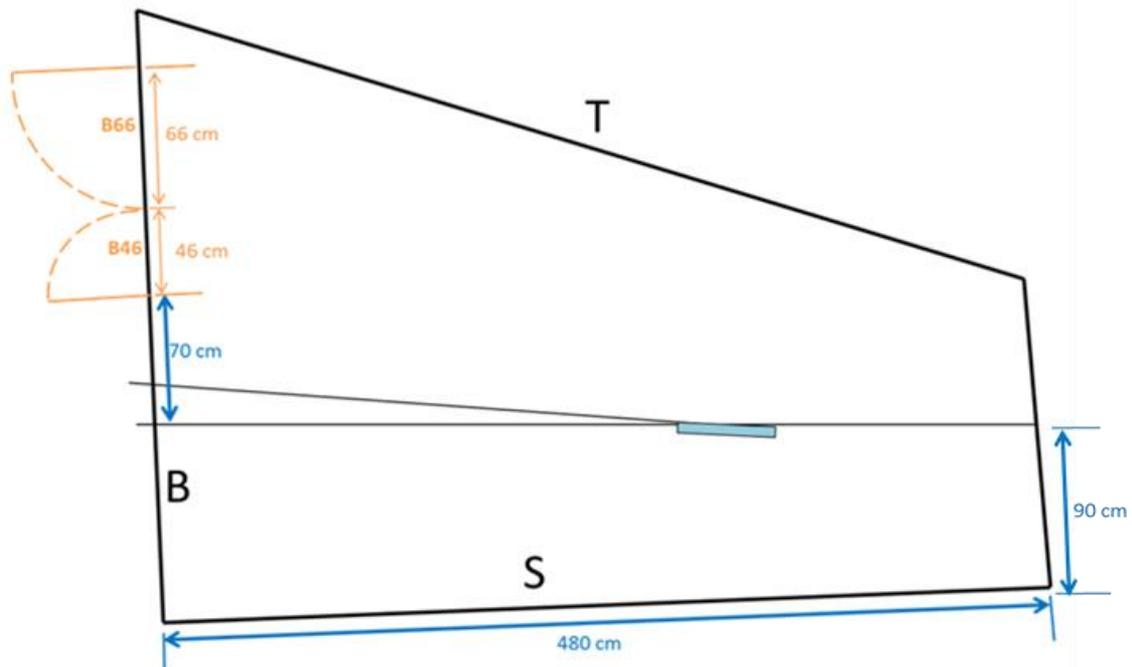
Fig. 1- Schematic layout of the LOREA optical hutch
