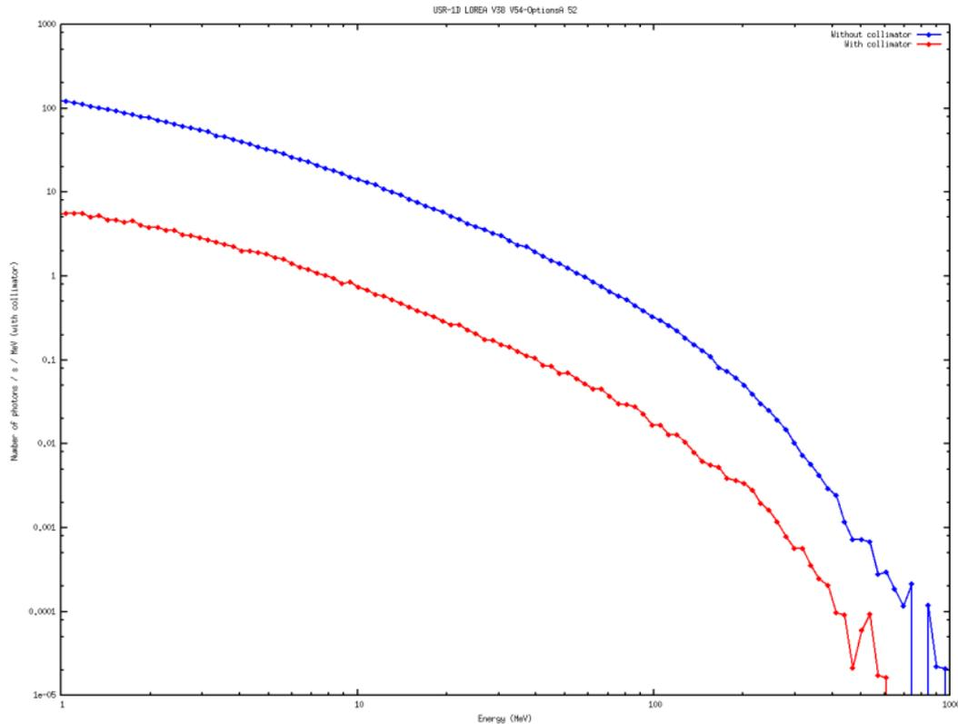
Fig. 7 - Transmitted scattered bremsstrahlung spectrum through the beampipe hole in the backwall (Photons / s / MeV); blue curve: no collimation; red curve: double collimator
