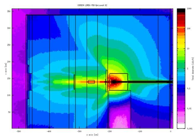
Fig. 5 - Vertical profile at the beam axis position of the total dose rate map (in  $\mu\text{Sv/h}$ ) from scattered bremsstrahlung
