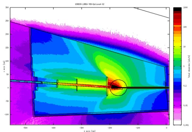
Fig. 4 - Total dose rate map (in  $\mu\text{Sv/h}$ ) from scattered bremsstrahlung
