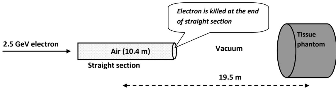
Fig.2 – Schematic of unshielded gas bremsstrahlung dose estimation in water phantom.
