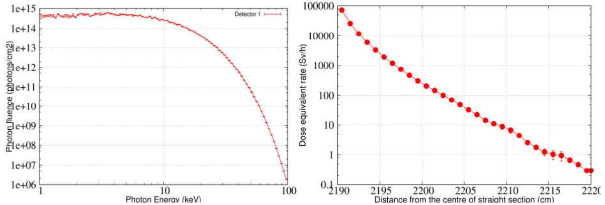
Fig-8: Synchrotron radiation spectrum (L) and the depth dose profile (R) inside tissue phantom for 200mA stored current in Indus-2
