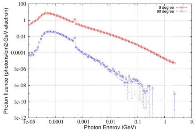
Fig.5 - Scattered gas bremsstrahlung spectra from pre-mirror in 0 and 90-degree direction
