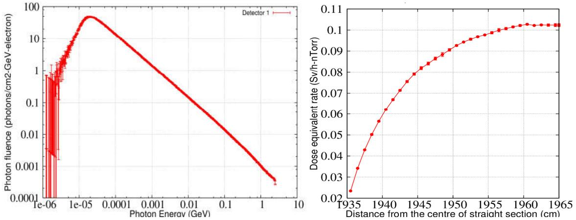
*Fig.3- Gas bremsstrahlung energy spectrum (L) and the depth dose profile (R) inside tissue phantom due to 2.5 GeV electrons passing through 10.4 m straight section*
