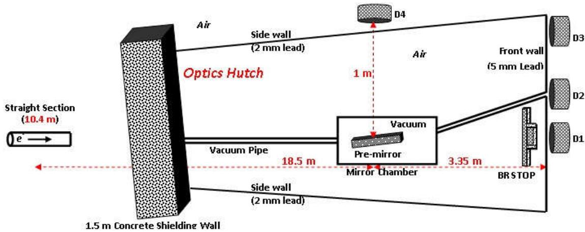
Fig.7- Geometry used for bremsstrahlung dose evaluation outside hutch area.
