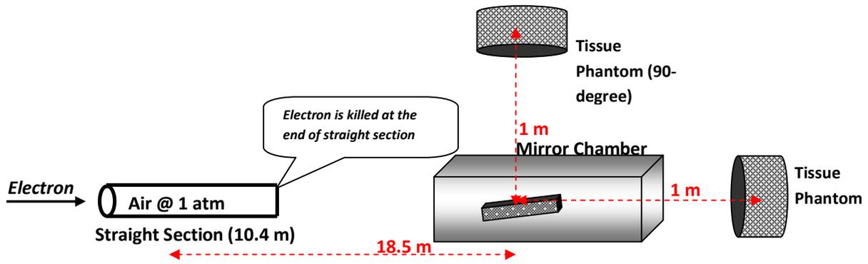
Fig.4- Geometry used for bremsstrahlung dose evaluation in 0 and 90 degree from the mirror
